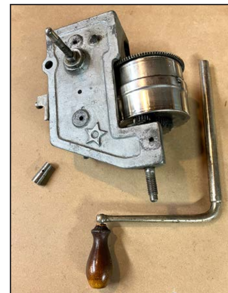
4. The output shaft (upper left), tapered sleeve (removed, left) and hand crank of a motor.
