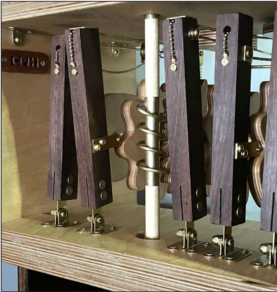
8. The worm gear and cam followers in the completed automaton.
