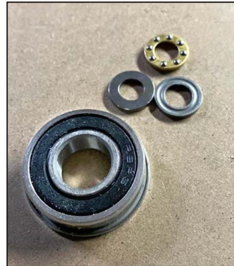
6. The \frac{1}{2} " I.D. and 1\frac{1}{8} " O.D. ball bearing. The smaller parts comprise a three-part thrust bearing with a \frac{1}{2} " O.D..
