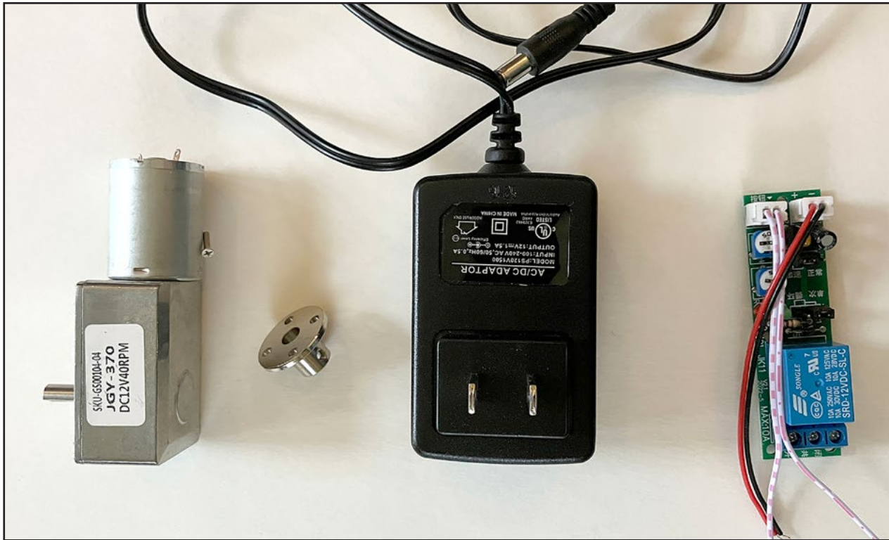
2. Motor, motor flange, 12-volt charger, and timer.
