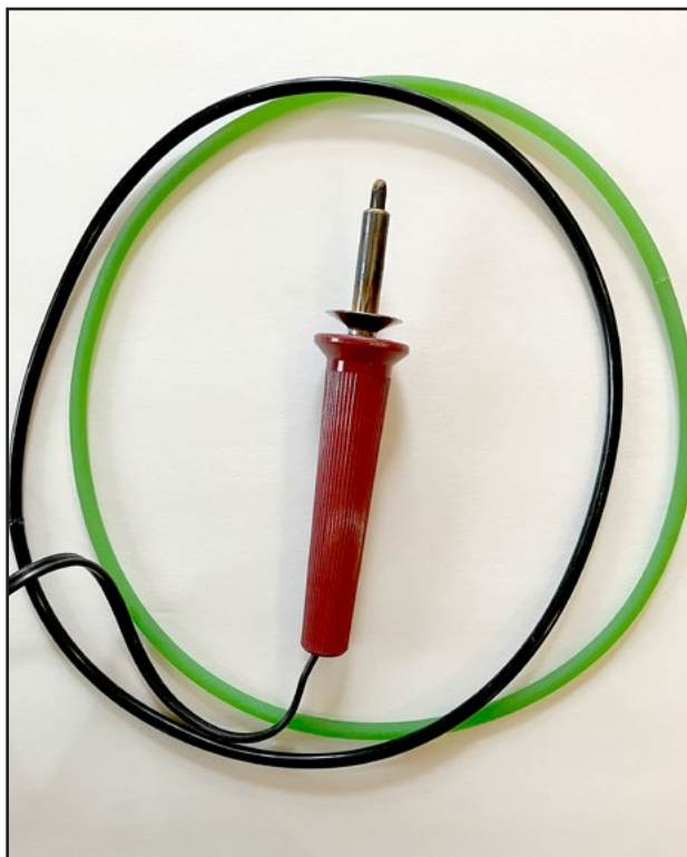
9. Polyurethane drive belts and a soldering iron with a beveled tip for joining cut ends.
