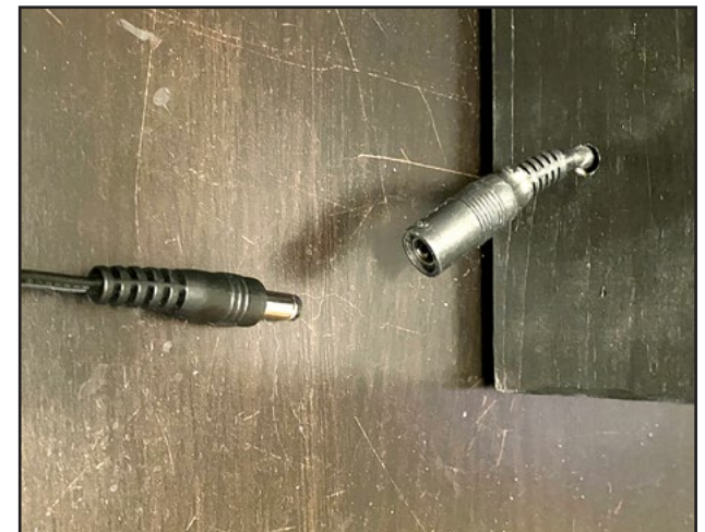
4. The charger's electrical connector, located outside the motor box.
