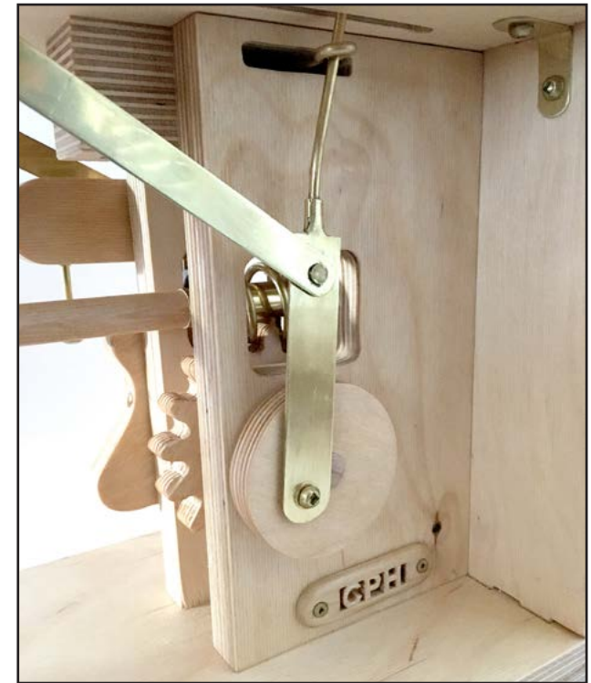
8. The final cam lever, with the pivot point between the follower and the load, proved to be a better solution.
