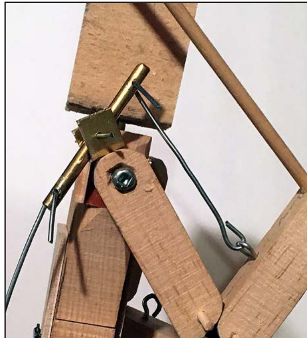
3. A prototype knight with a lever on his shoulder to control his sword arm.
