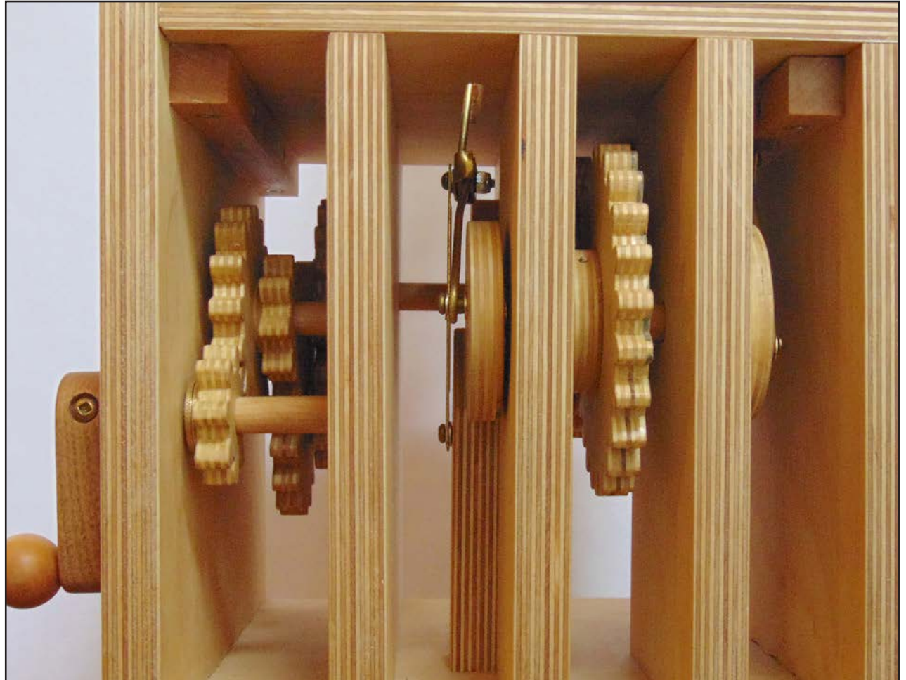
6. The Swordsman mechanism has three eight-tooth and three 16-tooth gears to step the rotation down to 8:1. With the Knights Battle , a 16-tooth gear on the crank and an eight-tooth gear on the driveshaft initially step the rotation up to 1:2 before stepping it down again to 8:1 and 9:1 with the worm gears.
