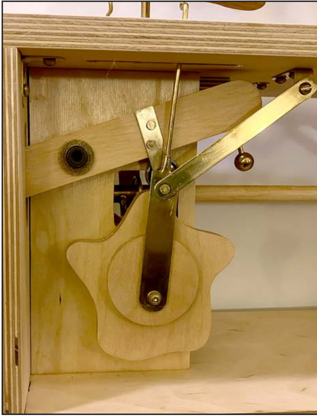
9. The control rod for torso rotation pokes out of the slot at the top of the photo.
